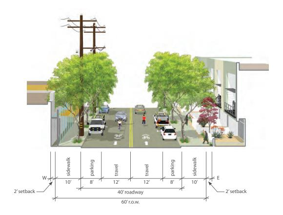
Improvements to First Street between Hubbard Avenue and Harding Street are intended to create a more inviting pedestrian, bicycle, and vehicular connection between the Metrolink Station and Maclay Avenue's "main street" and the Civic Center. Improvements occur within the existing right-of-way and curb-to-curb widths and consist primarily of the introduction of street trees and street lights. Improvements must incorporate the following:
