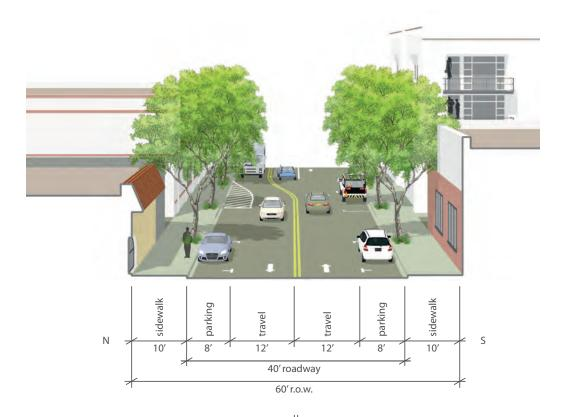
Improvements to Maclay Avenue between San Fernando Road and Pico Street within the existing right-of-way and curb-to-curb widths and consist of re-striping the travel lanes in order to introduce convenient on-street parking in front of Downtown stores and restaurants as well as to provide a buffer between vehicular traffic and the sidewalk. Streetscape improvements include the introduction of street trees and street lights. Improvements must incorporate the following:
