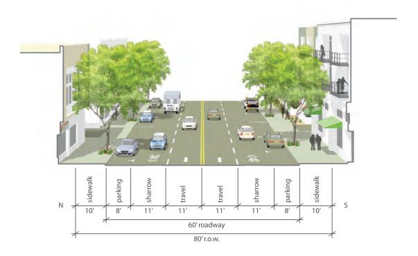
Improvements to San Fernando Mission Boulevard Road occur within the existing right-of-way and curb-to-curb widths and consist of re-striping the travel lanes in order to introduce convenient on-street parking in front of Downtown stores and restaurants as well as to provide a buffer between vehicular traffic and the sidewalk. Streetscape improvements include the introduction of street trees and street lights. Improvements must incorporate the following:
