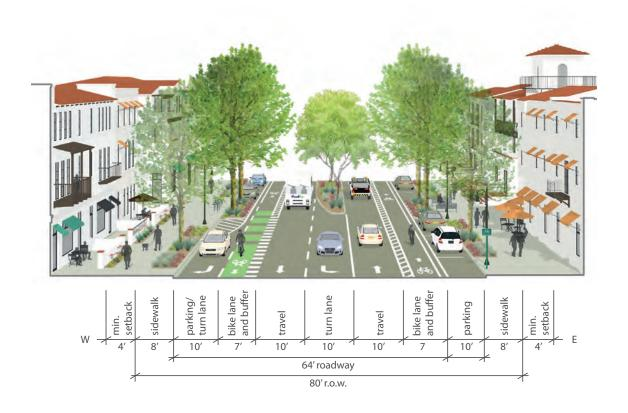
Since traffic loads along Truman Street between San Fernando Mission Boulevard and Hubbard Avenue, an alternative configuration could consist of one lane and a Class II bike lane in each direction separated by a center turn lane or landscaped median. Improvements occur within the existing right-of-way and curb-to-curb widths. Improvements must incorporate the following:
