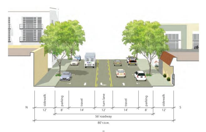
Improvements to Maclay Avenue between Truman Streets and San Fernando Road occur within the existing right-of-way and curb-to-curb widths and consist of re-striping the travel lanes in order to introduce convenient on-street parking in front of Downtown stores and restaurants as well as to provide a buffer between vehicular traffic and the sidewalk. Streetscape improvements include the introduction of street trees and street lights. Improvements must incorporate the following:
