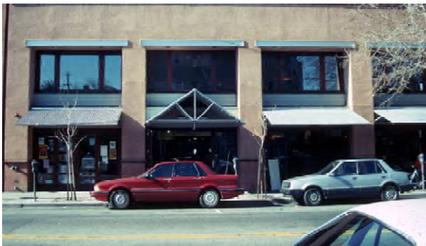
Subdivision can be created by using vertical piers to interrupt the length of a facade.
