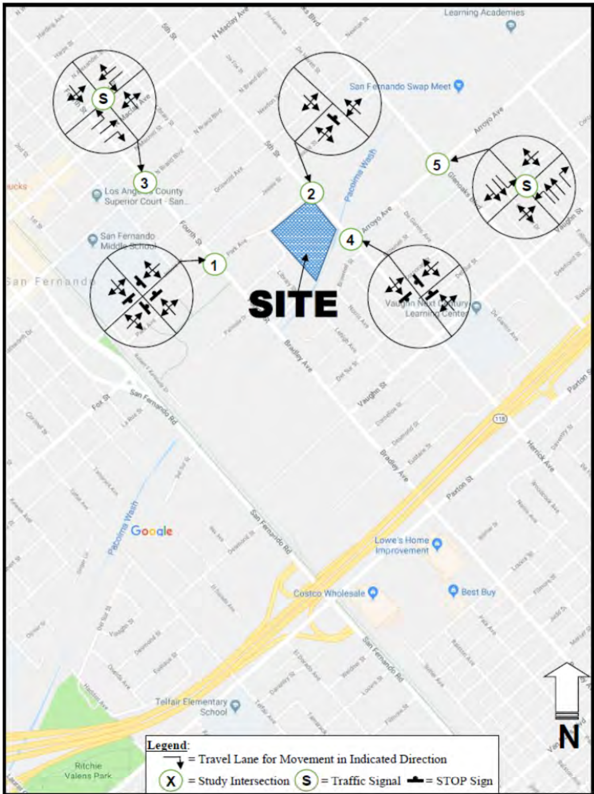
EXHIBIT 3-7 EXISTING LANE CONFIGURATION AT KEY INTERSECTIONS SOURCE: CROWN CITY ENGINEERS
