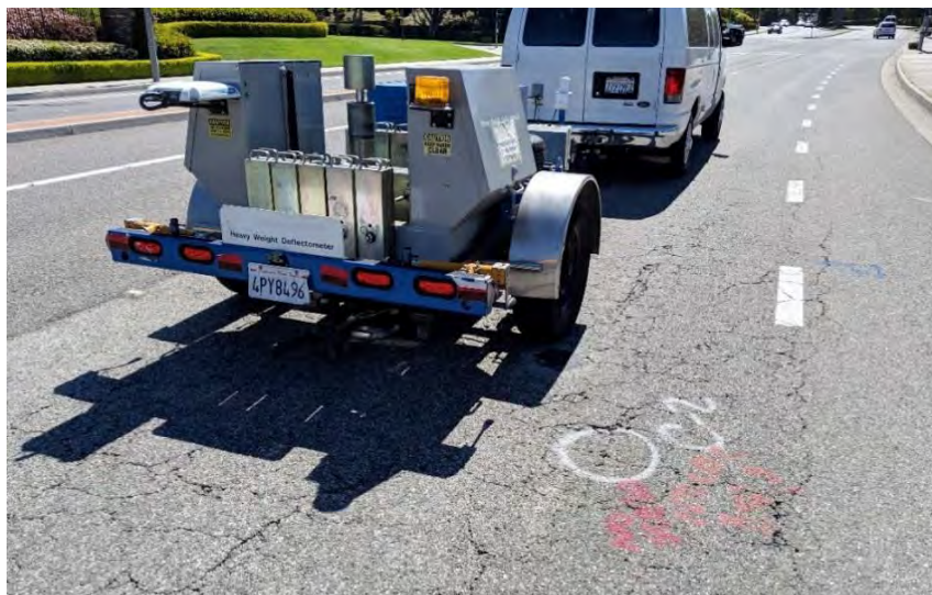
Photo 6: Pavement deflection testing being performed at coring location C-2 within area of medium-severity alligator cracking on Ford Road.
