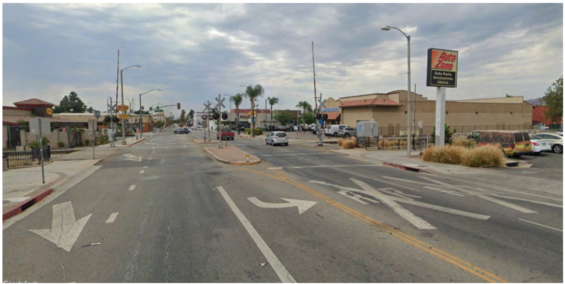
Image 24. Without crosswalks on the trail, users must take a detour to the nearest intersection, making the route less convenient and safe.
