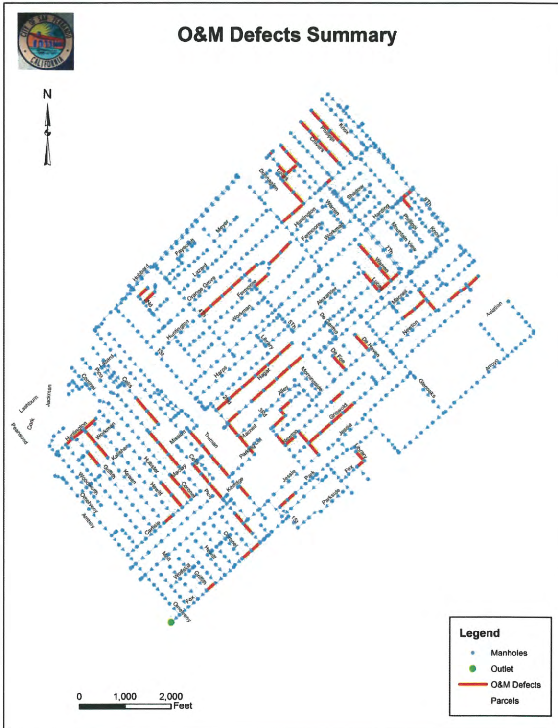
Figure 5-3. Sewers with Videotaped O&M Defects
