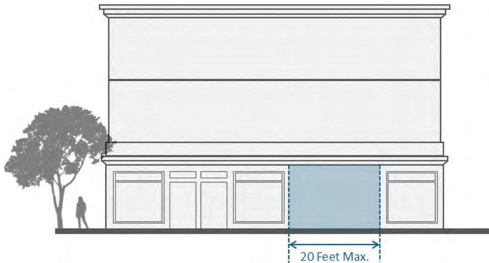
Figure. Blank Façade
