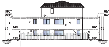
PROPOSED NORTH ELEVATION SCALE: 3/32"=1'-0"
