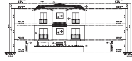
PROPOSED SOUTH ELEVATION SCALE: 3/32"=1'-0"
